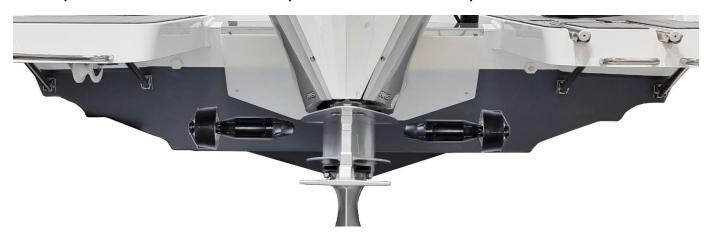
The brand new WS60 is a completely new way of mounting a stern thruster propeller system. When mounting conventional stern thrusters on boats with outboard motors or boats with stern drives, the motor / stern drives is in the way of get free water flow to both sides.
