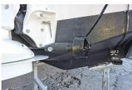
Engine: 2600w 3-phase direct-drive water-cooled.
